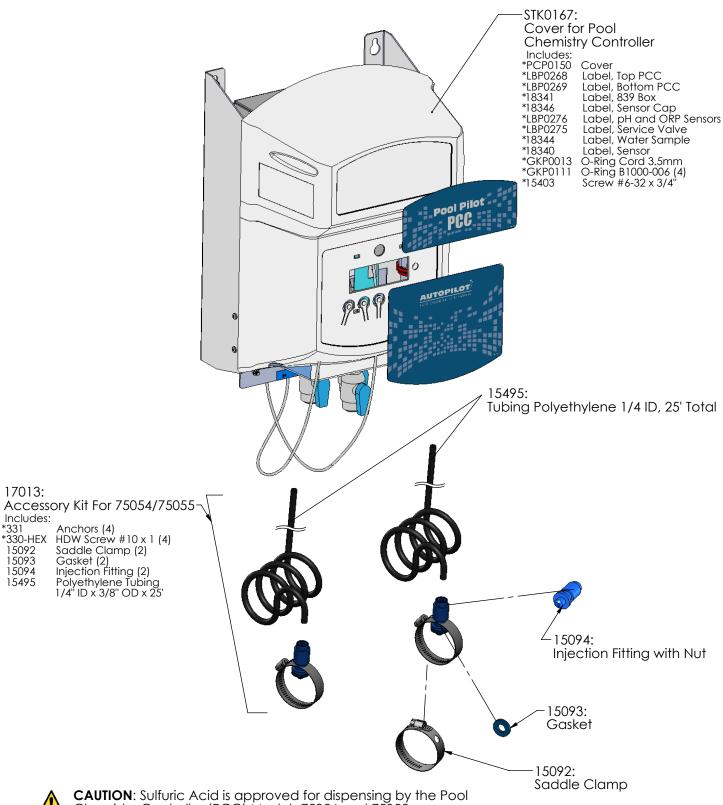
Chemistry Controller (PCC) Models 75054 and 75055. Muriatic/Hydrochloric Acid is **NOT** approved for dispensing by the PCC and will void warranty coverage if dispensed by the PCC.
